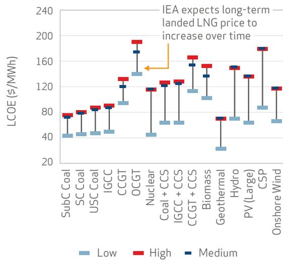
SubC Coal: Subcritical Coal; SC Coal: Supercritical Coal, USC Coal: Ultra-supercritical coal; IGCC: Integrated Gasification Combined Cycle; CCGT: Combined Cycle Gas Turbine; OCGT: Open Cycle Gas Turbine; PV: Photovoltaic; CSP: Concentrated solar power
