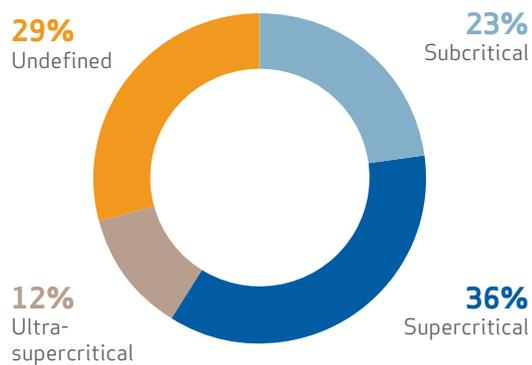
Recent estimates indicate a \$490 million capital cost difference between a subcritical and ultra-supercritical option for 1GW plant in ASEAN. While the ultra-supercritical option has a higher upfront expenditure, the emission rate is a quarter lower. Moreover, the increased efficiency of the plants mean fewer tonnes of coal consumption and therefore long-term lower operating costs.
