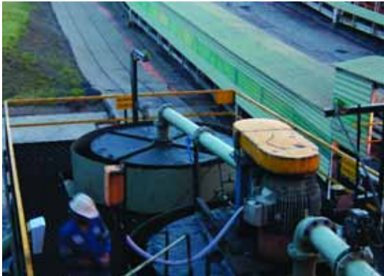
Froth flotation cells at Goedehoop Colliery are used for fine coal beneficiation. Photograph courtesy of Anglo Coal.
